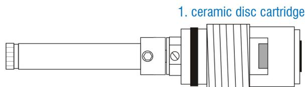
4. Ensure that the disc is in the closed position and then fit handle to align.
